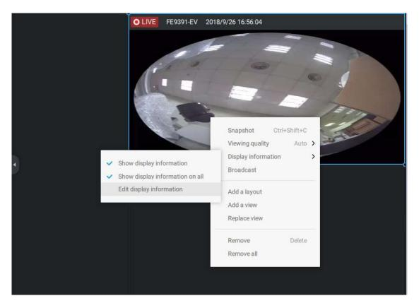
Select the checkboxes to determine what kind of text overlay will display on view cells. Note that you can place the overlay either on top or at the lower screen. Simply click and drag an overlay item to a preferred location. When done, click the Apply button.
