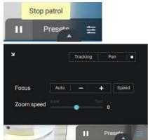
The PTZ settings tab allows you to enable PTZ Tracking and the Pan functions. You can also adjust the Zoom and Focus speed, or manually adjust the focus. Please refer to the camera User Manual for more information about these functions.
